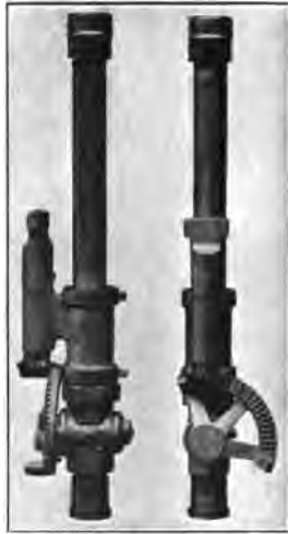
FIG. 65.—Pitometer Street Connection.
